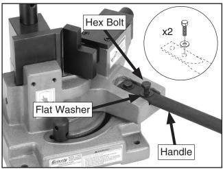
Figure 5. Attaching handle.
